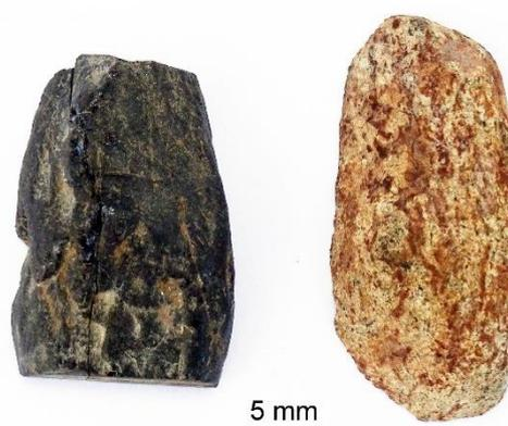
**Fig. 2:** Fergusonite specimens from Kolonna (left) and Masimbula (right), after being cut in half. Note that upper and lower tips of the Kolonna sample were cut off for analysis during a previous research (Prame et al., 2014)
